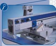
• 'Tool-free' front and rear stroke length adjustment - with no wires.
